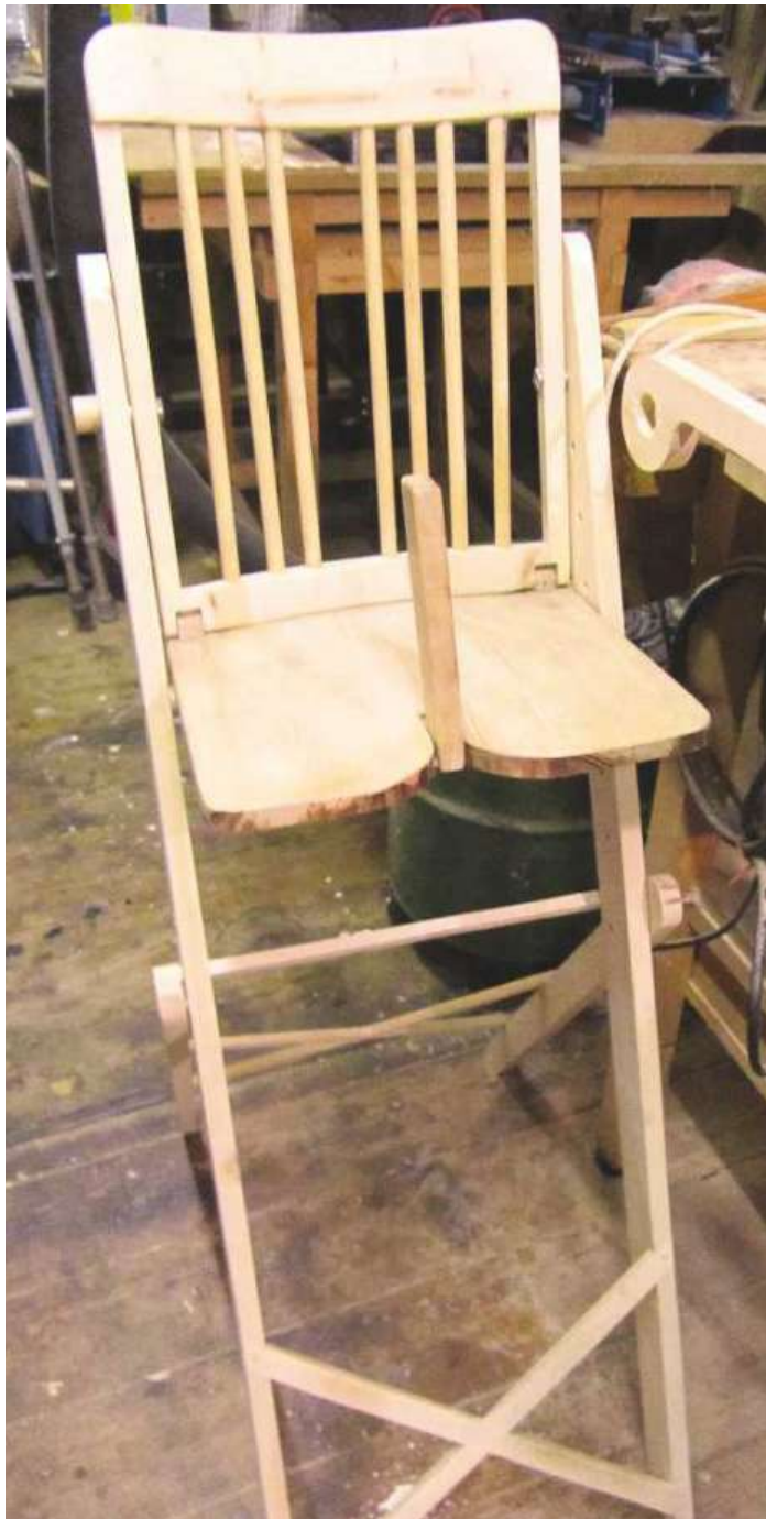
◀ Pic.6 The legs, which fold flat, are braced with thin struts and stop-bars. The struts are held together with halving joints, and pegged and glued to the legs
